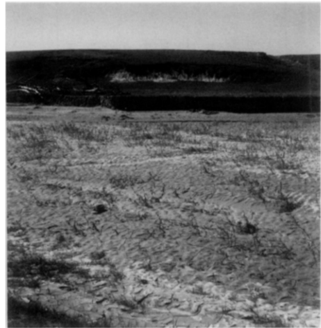
FIG. 7. Photographs of cross section 6 taken in 1957 (A) and 1967 (B). Over 2 m of sediment has filled in this cross section in the 14-yr interval between the 1957 and the 1971 surveys. Downstream is to the left in both photos.
